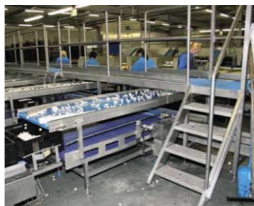
After any sub-standard examples have been removed, the mushrooms are placed into crates.
