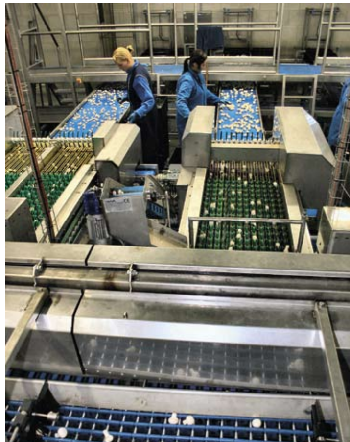
In the foreground the mushrooms are graded on the new cap diameter sorting system, followed by cutting and the removal of sub-standard
