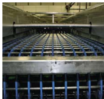
The innovative rod system with lines of flexible 'trains'. The cap diameter can be set in 5 millimetre increments.
