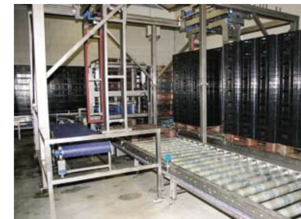
The Nawi logistic system ensures an even flow of crates and labels the produce.
